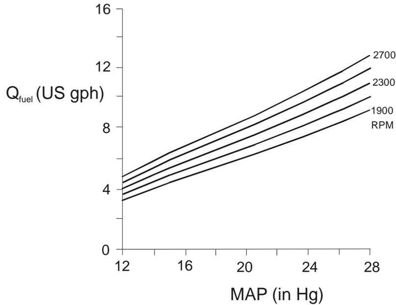
**Fig. 4.7(c) Fuel consumption rate in U.S. gallons per hour as a function of MAP and engine shaft speed, Lycoming O-320-A2B.**
